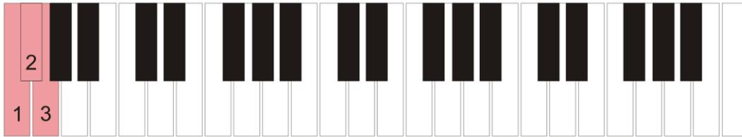
**Reset** (hold keys 1, 2, and 3 to Reset the configuration at Power On)
