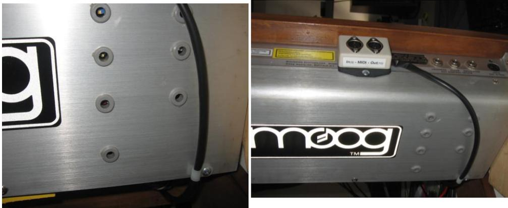
Use the second supplied longer screw to fit the cable clip, then route the cable down and through the hole in the case along with the other cableforms.
